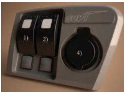
Kuva 8. SUIV 5700 SR CC, 5700 SR DUO, 5080 SR, 5050 SR DUO, 4750 SR DUO, 4650 SR, 4250 SR, Meri-Palta CC ja Meri-Palta 525 mallien kytkinpaneeli.
