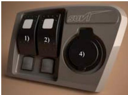
Kuva 7. Suvi 5700 SR CC, Suvi 5700 SR Duo, Suvi 5050 SR DUO, 5050 SR UNO, 5050 SR UNO CC, 4750 SR DUO, 4650 SR, 4250 SR, Meri-Palta CC ja Meri-Palta 525 mallien kytkinpaneeli.
